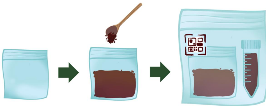
Figure 8: Procedure to collect soil sample for off-site heavy metals and nutrients assessment
