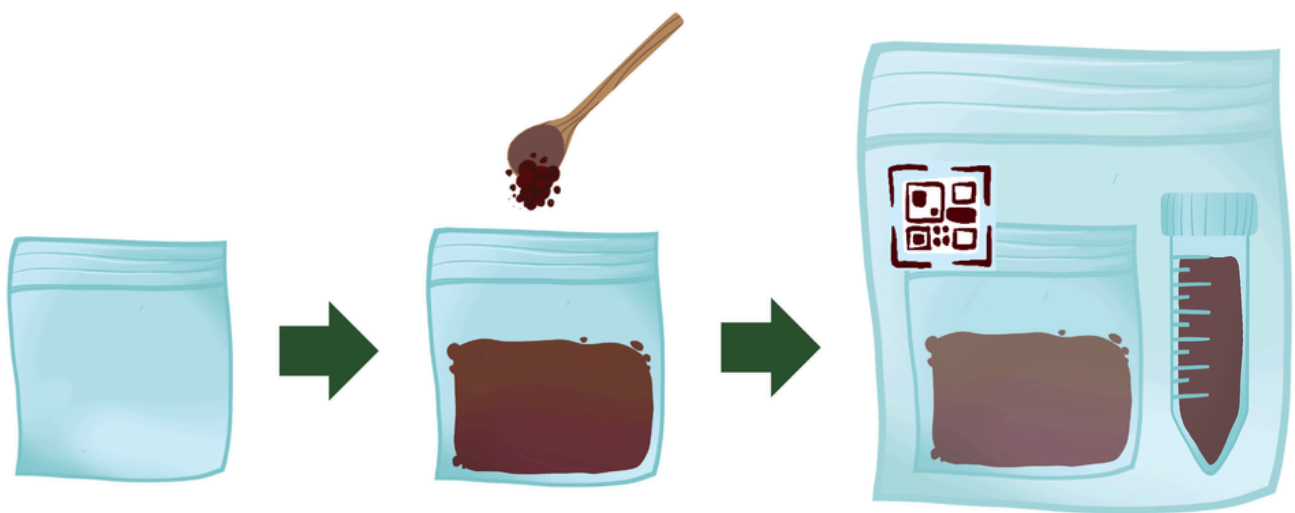
Figure 8: Procedure to collect a soil sample for off-site heavy metals and nutrients assessment
