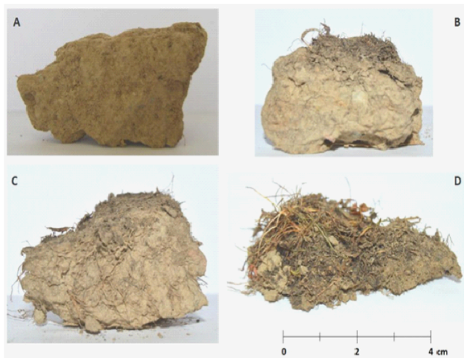
Examples of different soil structure types. A: massive, B: prismatic, C: blocky, D: granular
